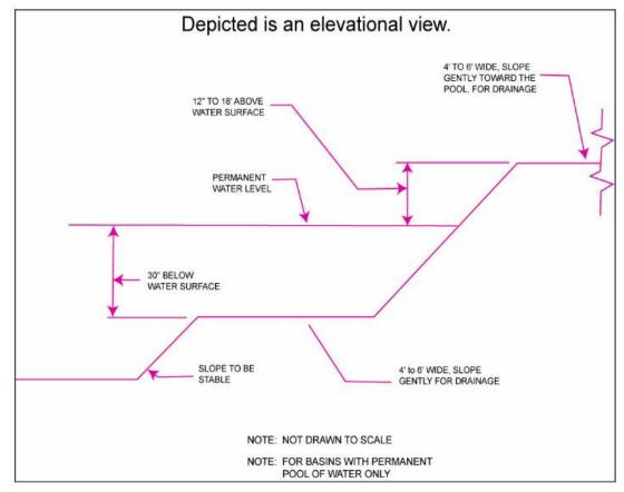
D. Illustration of Safety Ledges in a New Stormwater Management Basin.
